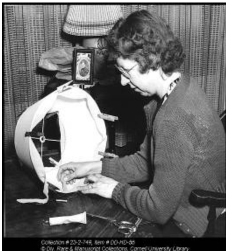
Caption reads: "Using a flexible tool such as a wooden ice cream spoon, force the material over each ring and down between the ring and the paper lining." Photo courtesy of Elmira Sunday Telegram. Date: 1950's Source: College of Human Ecology, Cornell University Library: Rare and Manuscript Collections < http://he-
